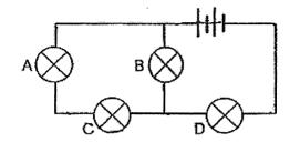
Which of the following bulbs, A, B, C or D, when removed, will cause none of the bulbs to light up?
