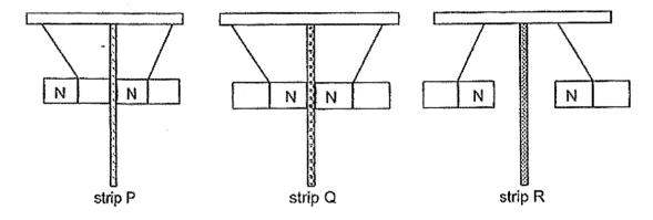
Which of the following strip(s) is/are definitely made of a magnetic material?
