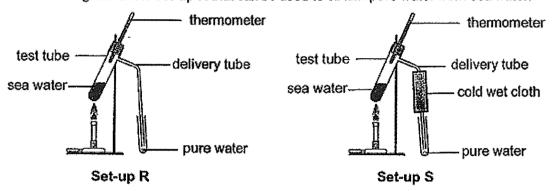
Rahman suggested wrapping the delivery tube with a cold wet cloth, as shown in set-up S, will increase the amount of pure water collected in the test tube over a period of two minutes.
