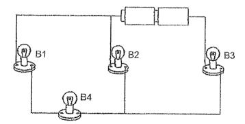
One bulb fused and none of the bulbs could light up. Which of the bulb(s) could have fused to cause this result?
