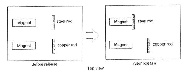
After both rods were released, the steel rod was observed to roll towards the magnet, but the copper rod stayed in the same position.
