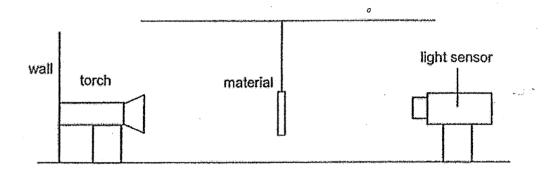
He placed each material between the torch and the light sensor and recorded the amount of light detected by the sensor. The table below shows his results.
