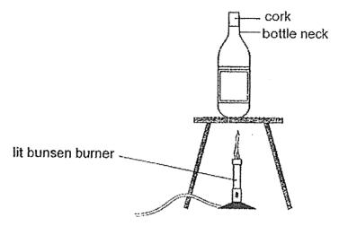
After 2 minutes of heating, the cork was seen moving up the neck of the bottle. Then, Tom could remove the cork from the bottle.
