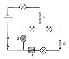
When the switch is closed, only 3 bulbs lit up. Which one of the materials, P, Q, R or S is an electrical insulator?
